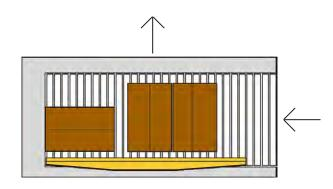
The row conveyor is cycled to receive the product and can run for additional time to create a gap prior to next product entrance.
