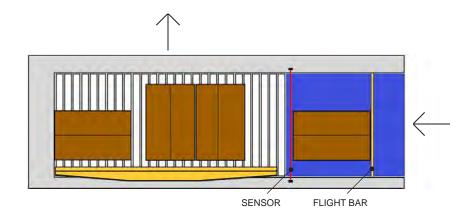
Positive indexing combines known product dimensions with a flight bar squaring solution. Product dimensions are integrated in load build programming, and initiate several palletizer operational parameters through positioning feedback drives. Product dimension data is relevant for positive index row building technology.
